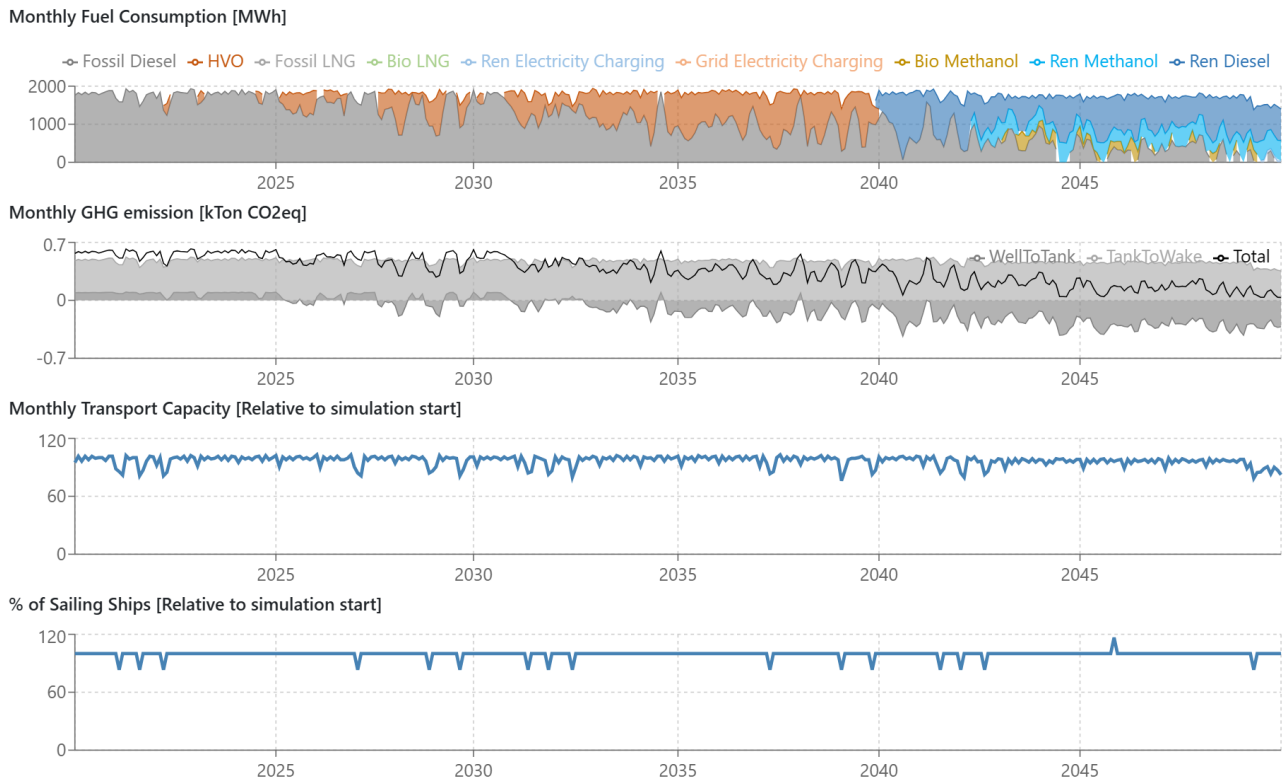
Figure 14: Development energy mix, GHG emissions, transport capacity and sailing 135 metre motortanker vessels on route Antwerp - Rotterdam at Innovative early adopter scenario
